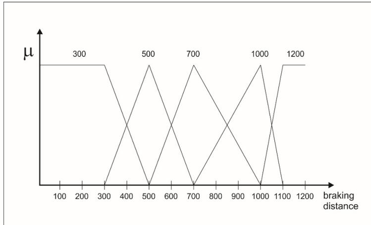
Figure 6. Membership functions for output variable  $y_1$  braking distance
