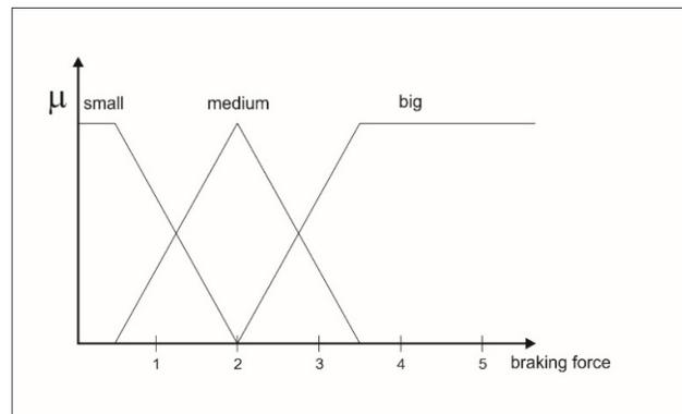
Figure 4. Membership functions for input variable  $x_3$  braking force
