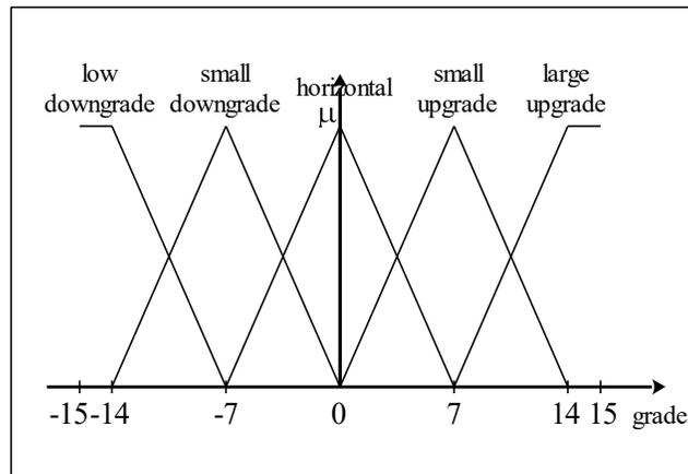
Figure 3. Membership functions for input variable  $x_2$  grade
