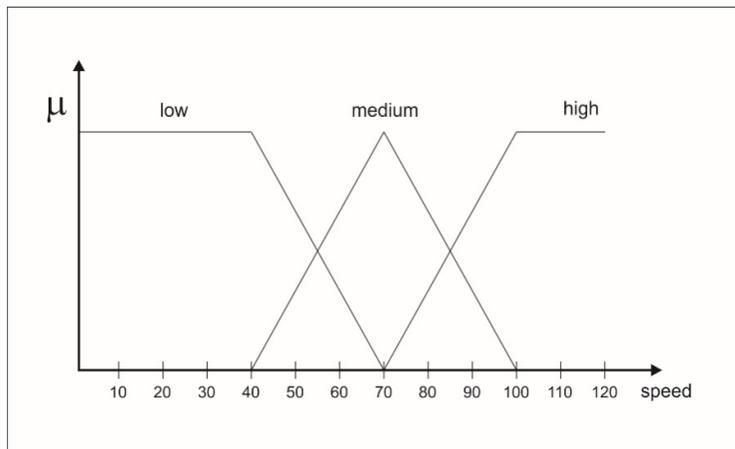
Figure2. Membership functions for input variable  $x_1$  train speed
