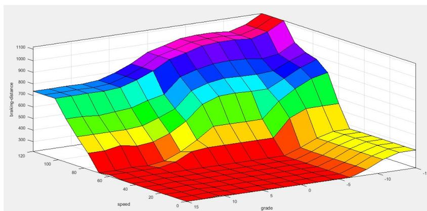
Figure 7. Surface viewer for input speed and grade and output braking distance
