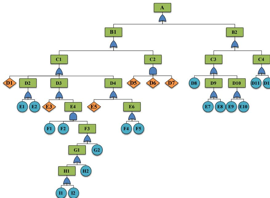
Figure 1. Fault tree of Westinghouse railway crossing
