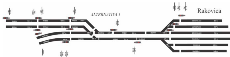
Fig. 2. Block section plan of part of the Belgrade node - junction G system
