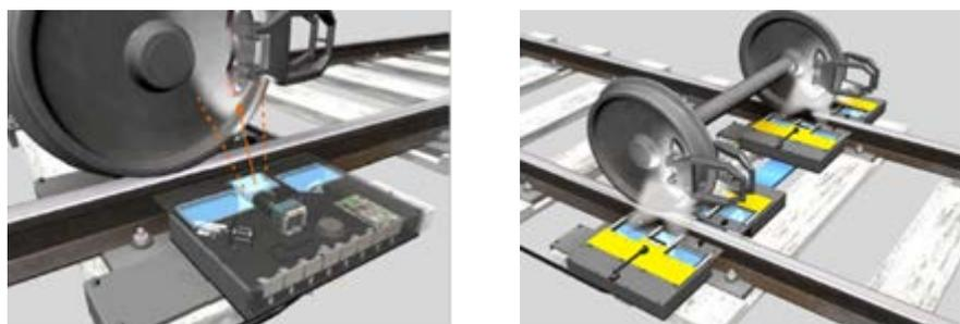
Fig.8. Measuring equipment for an axle set
