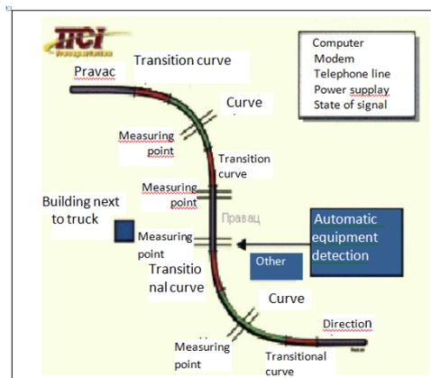
Fig.3. Measuring deflection points deflection in the "S" curve
