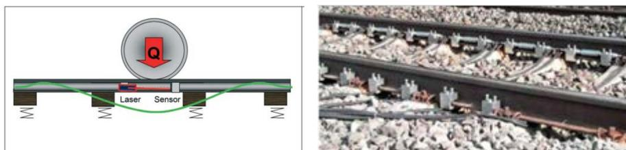
Fig.7. Schematic presentation of the principle of work of Lasca system
