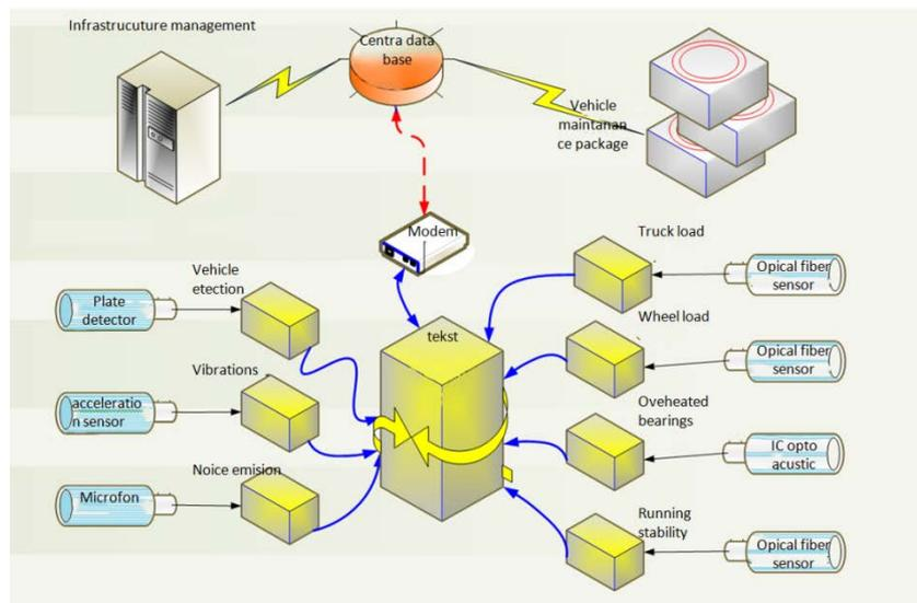
Fig.13. System measuring modules configuration
