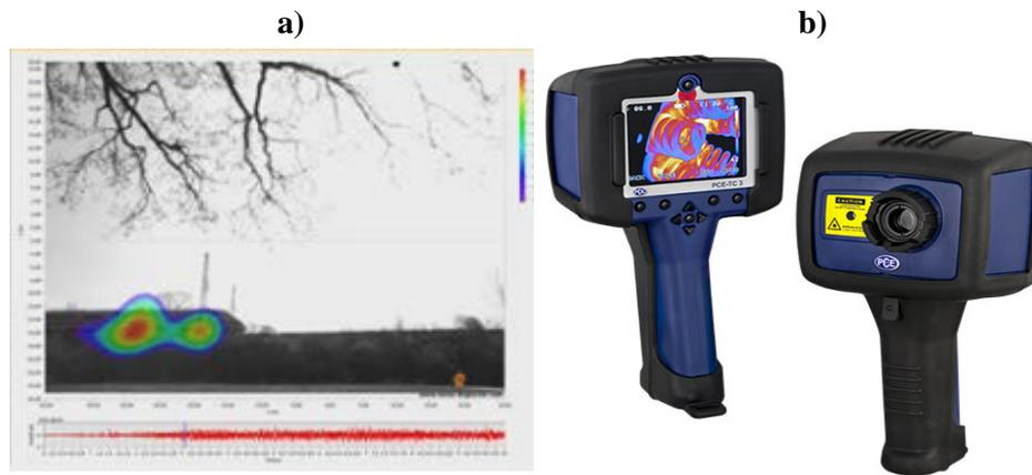
Fig.2. Measurement of temperature a) motor, b) thermo-vision camera
