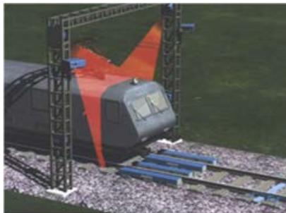
Fig.9. Device for determining the profile of the train
