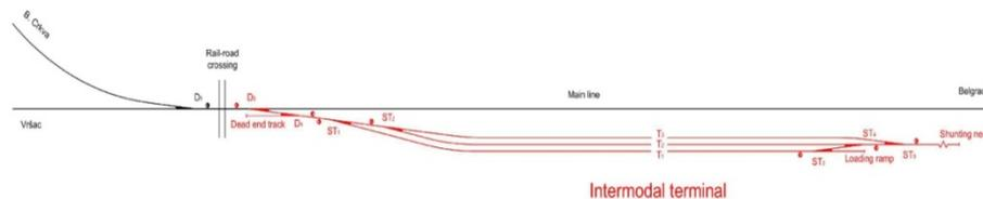
Fig.2. The layout of the rail-road transshipment yard
