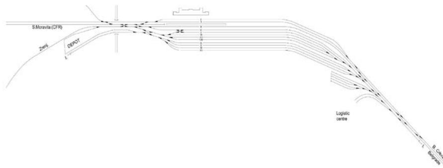
Fig.1. The reconstructed layout of Vršac railway yard
