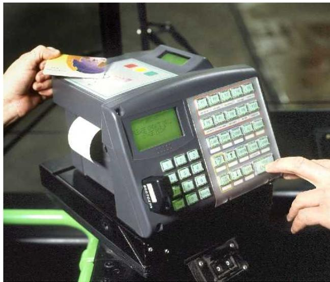
Fig.2.The appearance of units for sale of individual tickets in vehicle
