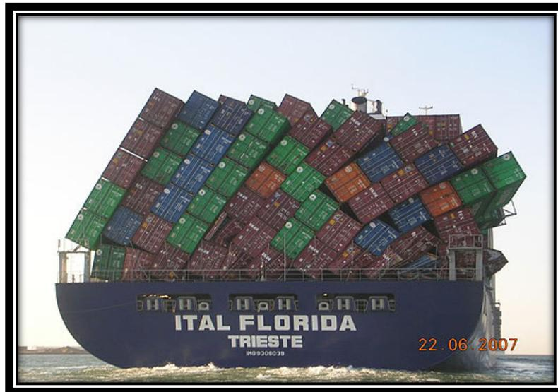
Fig.4. -Containers falling overboard during transport
