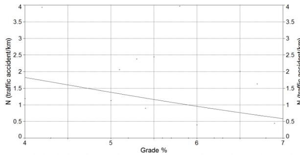
Fig. 2. The model of the dependence of the total number of accidents on the gradient
