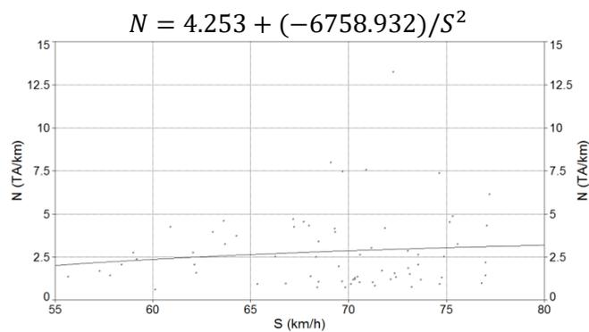
Fig. 9. The model of the dependence of the number of accidents on the speed
