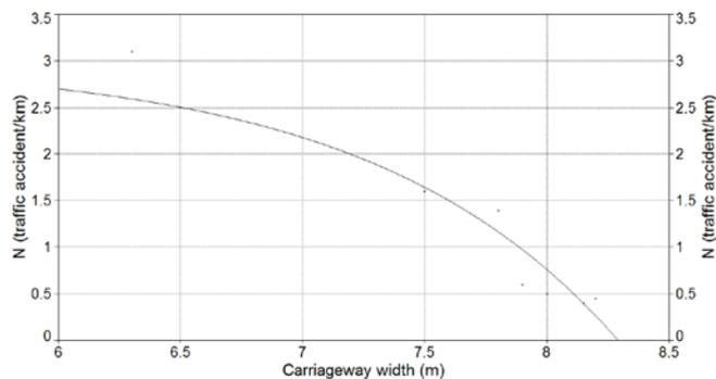
Fig. 3. The model of the dependence of the number of accidents on the carriageway width
