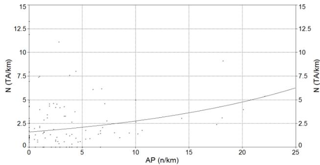
Fig. 9. The model of the dependence of the number of accidents on the access points
