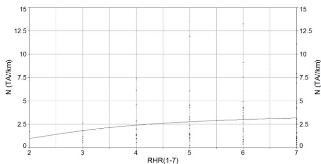
Fig. 4. The model of the dependence of the number of accidents on the roadside hazard rating
