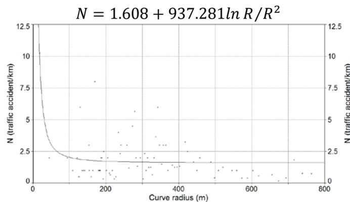
Fig. 1. The model of the dependence of the total number of accidents on the horizontal curve radius
