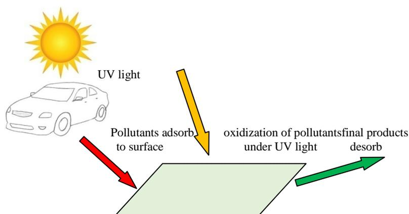
Fig.1. Illustration of the photocatalytic process
